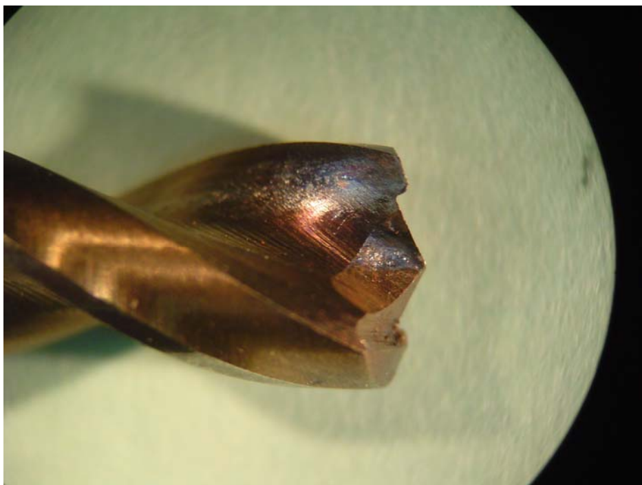
(Fig. 20) TG – higher magnification of burning on cutting edge – Minimal and no material roll over or melting present compared to competitor's figure number 17
