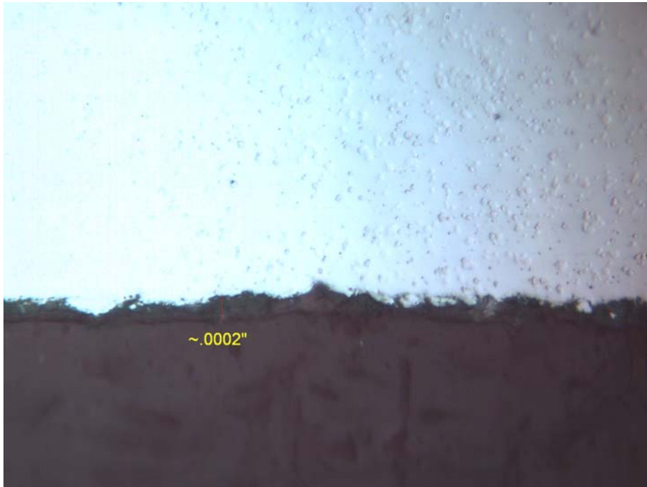
(Fig. 22) 1000x - TG surface – coating is ~.0001"
