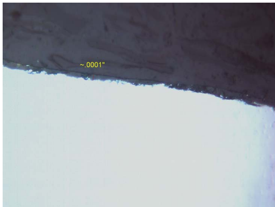
(Fig. 21) 1000x - 17/64 Surface – coating is ~.0001"
