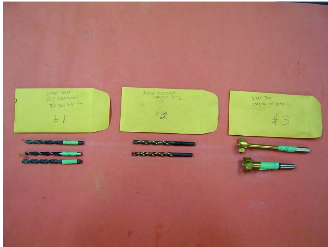
(Fig. 1) All seven drill bits tested for metallurgical properties after mechanical testing
