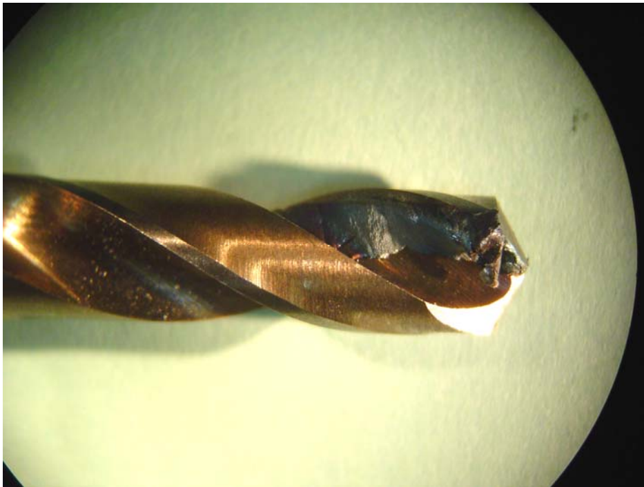
(Fig. 16) 17/64 – photo showing cutting edge. Note material build up on flute
